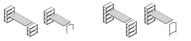
The table solution consists of a tabletop including traverse for single-sided and two-sided connection to profile and/or table leg.
